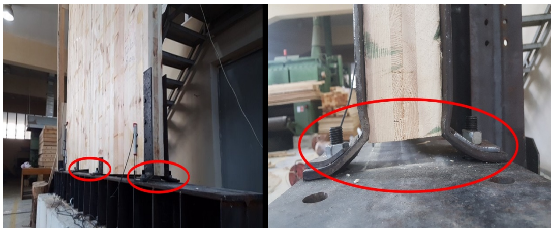
Figure 6. Failure modes of CLT shear walls
