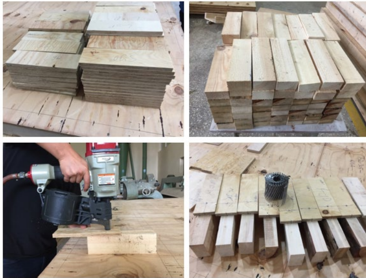
Figure 1. Preparation of specimens for lateral nail strength test
