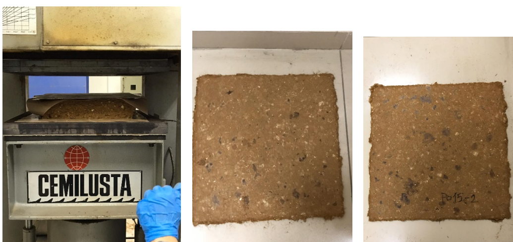
Figure 2. Production of mycelium based MDF
