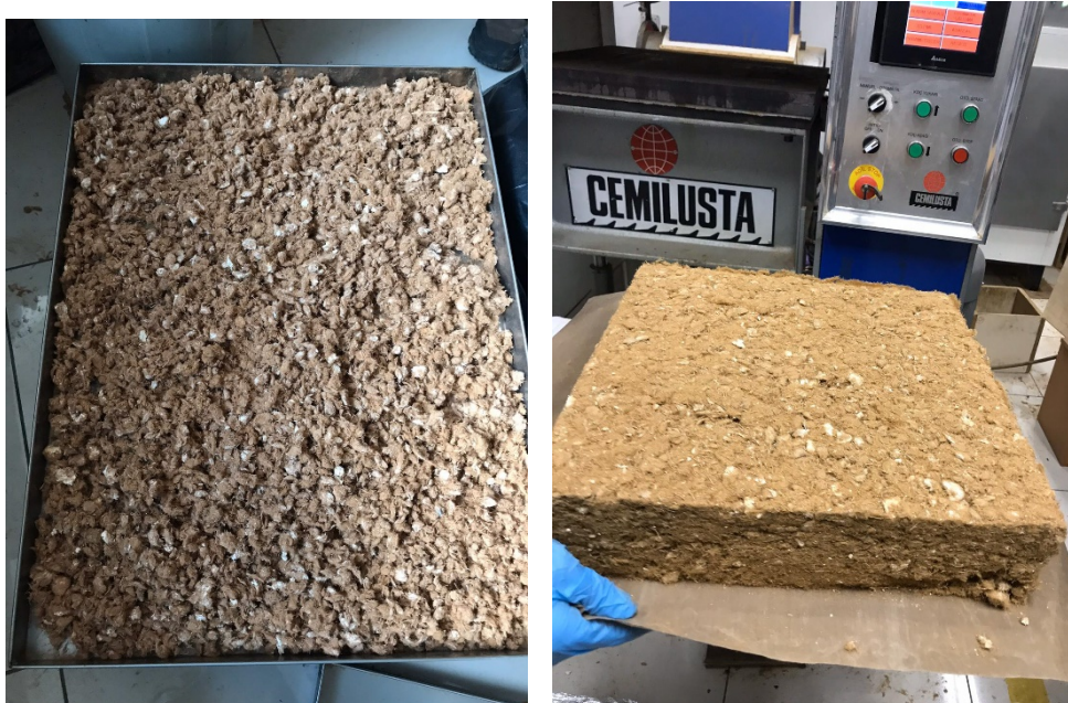
Figure 1. Preparation of mycelium based MDF
