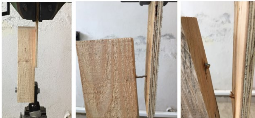
Figure 2. Lateral nail strength test setup and changes at the end of the test
