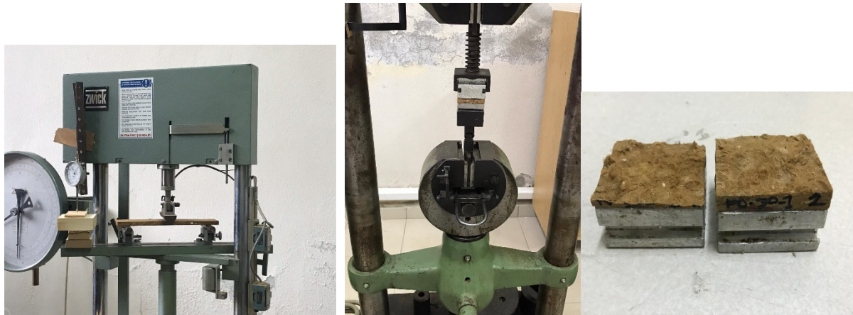
Figure 3. Mechanical tests of mycelium based MDF
