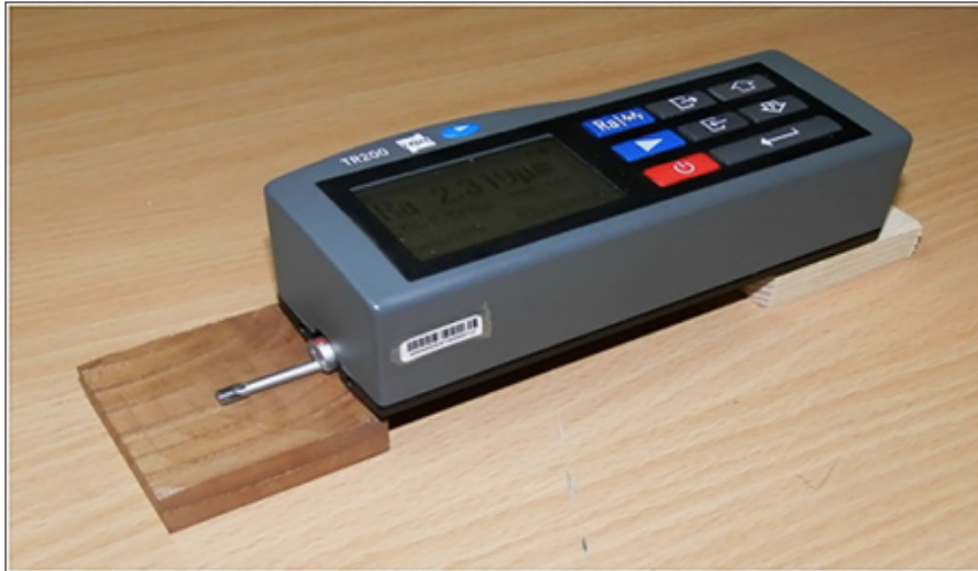
Figure 4. Stylus contact tester ( TR200 TIME, China ) for measurement of parameter R
