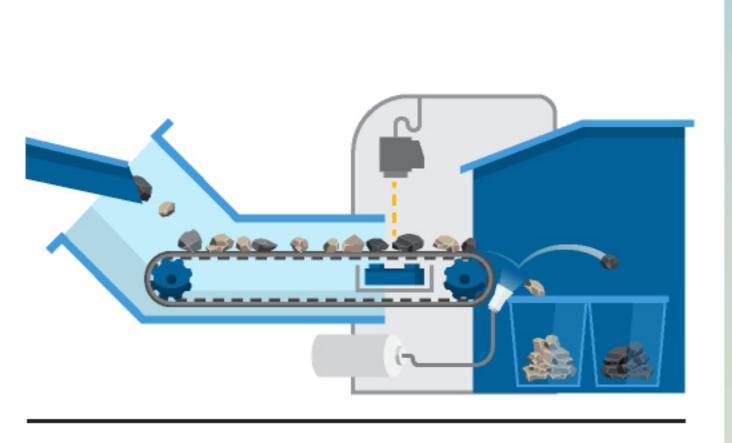
Ore sorting reduces the quantity of material that needs to be crushed and ground to unlock valuable minerals and metals, saving energy and resulting in less mine waste.
