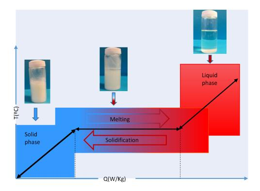
Figure 1. Heat storage mechanism in a PCM.
