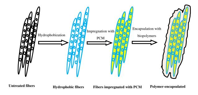
Figure 4. Schematic representation of incorporating PCMs into bio-fibers.
