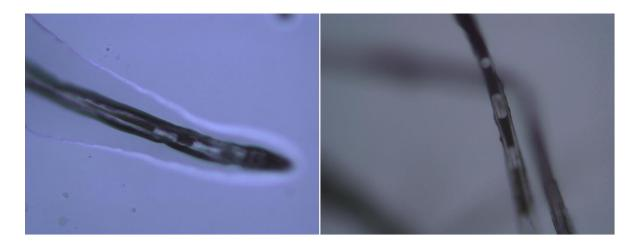
Figure 5. Microscopic images of BPCM into wood fibers.
